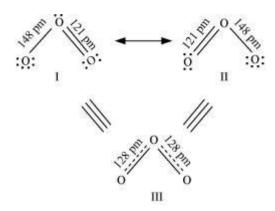
Here, I and II are resonance structures while III is the resonance hybrid.
